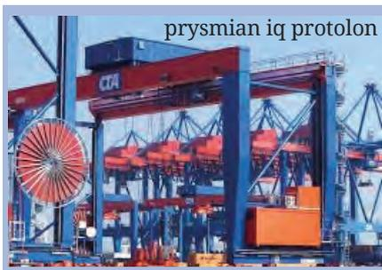
XLPE (cross linked polyethylene), using HPTE (high performance thermoplastic elastomer polypropylene based insulation). P-Laser insulated cables withstand increased operating temperatures by over 20 per cent, abiding to fluctuating demands in harsh environments. P-Laser cables production process utilises zero gas technology, reducing CO2 emissions by 1-tonne per km. Furthermore, degassing is no more required.”
